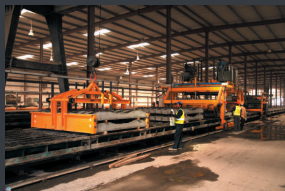
Sleepers ready for inspection
